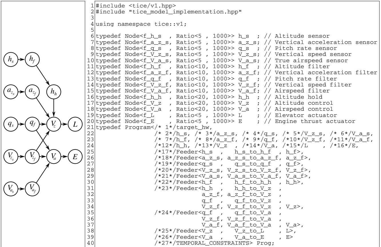
FIGURE 8 ROSACE's MATLAB/SIMULINK model expressed as Tice model (left) and its expression in Tice language (right).
